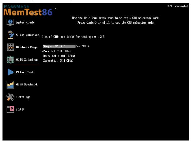
Single - specifies a single CPU core to test, and prompts the user to enter a valid CPU ID number
