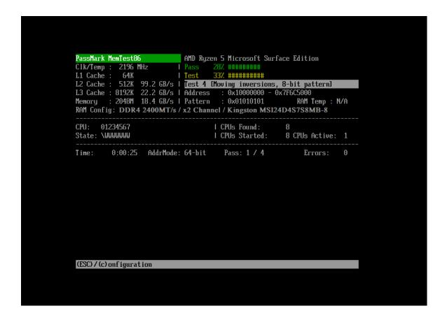
MemTest86 executes a series of numbered test sections to check for errors. The execution order for these tests has been arranged so that errors will be detected as rapidly as possible.
