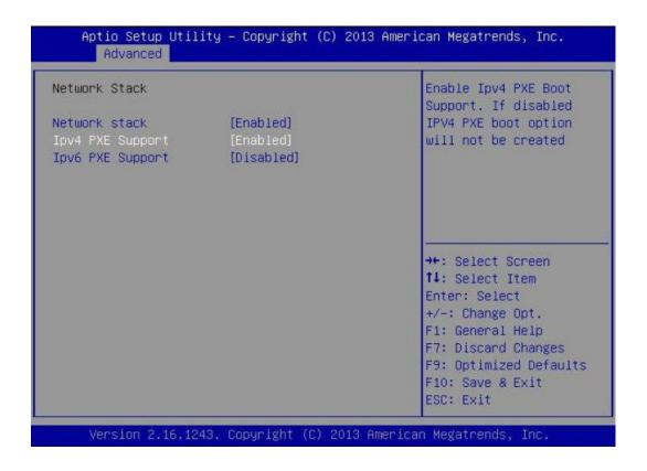
Once PXE support is enabled, ensure that the network PXE boot option is in the appropriate boot order.
