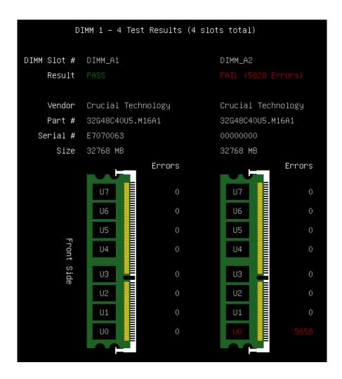
MemTest86 (Site Edition) further supports decoding of the individual DRAM chip in which the error occurred. The DRAM chip mapping (eg. U0...U7) can be defined with the configuration file parameter *CHIPMAP*. See Configuration File (*Pro version only*) for more details about configuration file parameters.
