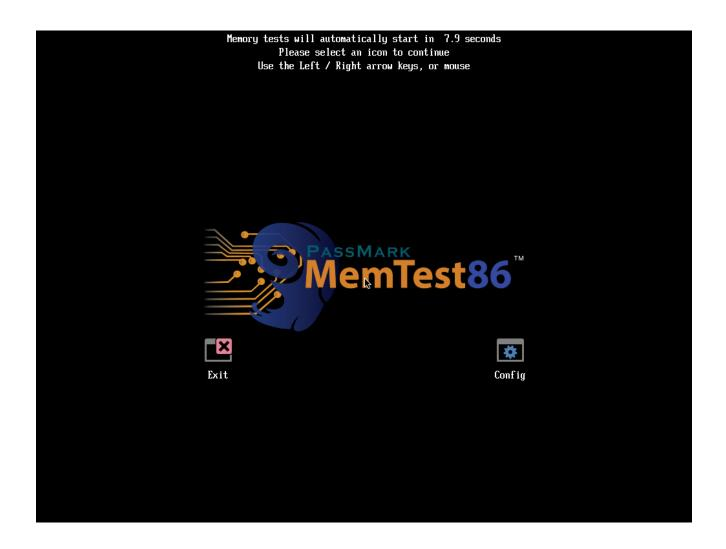
Selecting **Exit** shall allow the user to reboot, shutdown or exit MemTest86. To configure the memory tests, select **Config** and the main menu is displayed. The main menu allows the user to customize the memory test settings such as the specific tests to execute, address range to test and which CPU core(s) are used in testing.
